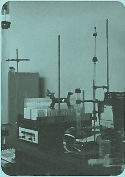
Fraction Collector and Ion Exchange Column — Toxin Purification
